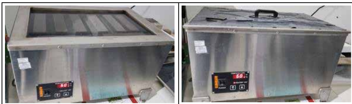
Figure 6-7 Immersion of mortar prisms in hot water at 60°C.
