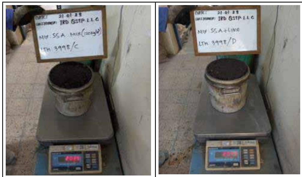
Figure 5-18 Fresh density testing of CBM mixtures
