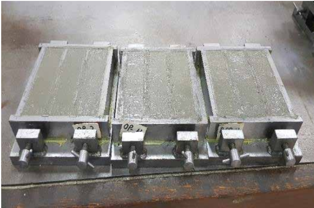
Figure 3-11 Casting of the fresh mortar prism specimens
