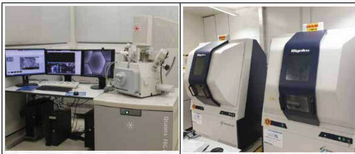
Figure 4-18 Quanta650FEG SEM (left) and Rigaku's SmartLab XRD (right) equipment
