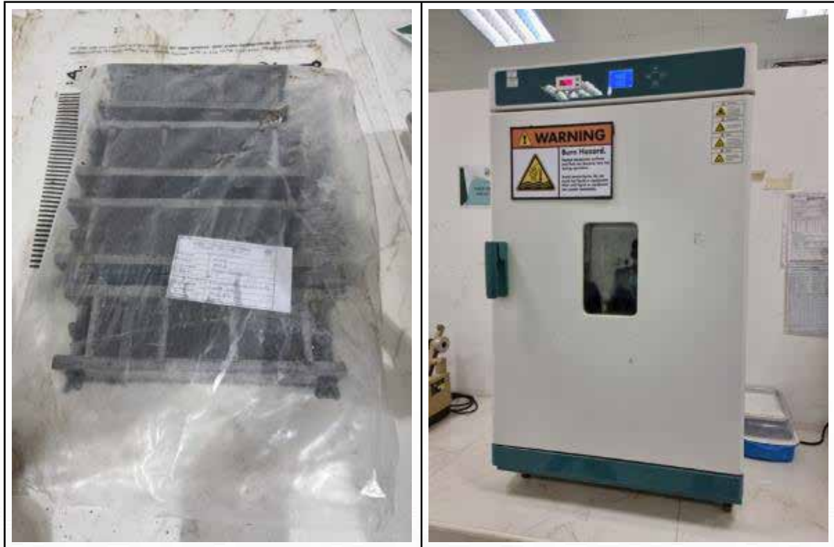
Figure 4-2 Sealed cube moulds and oven curing
