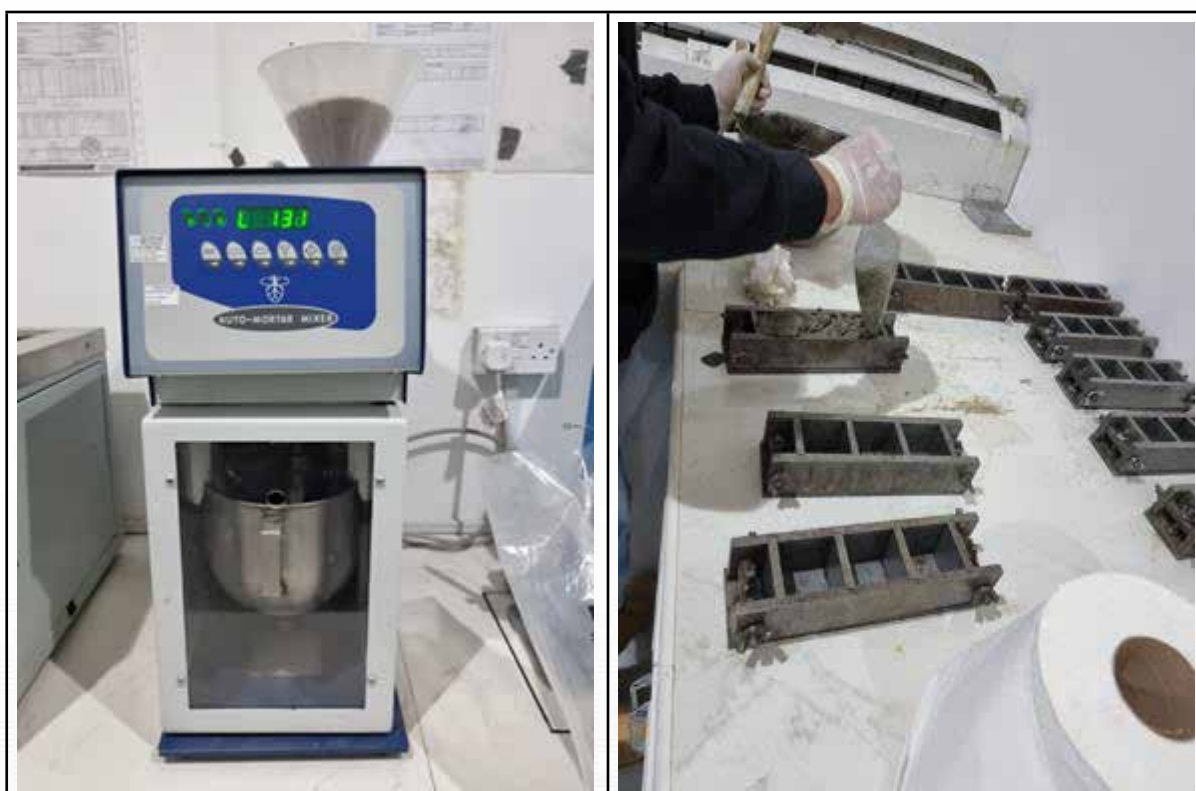
Figure 4-1 Mortar mixing and cube preparation
