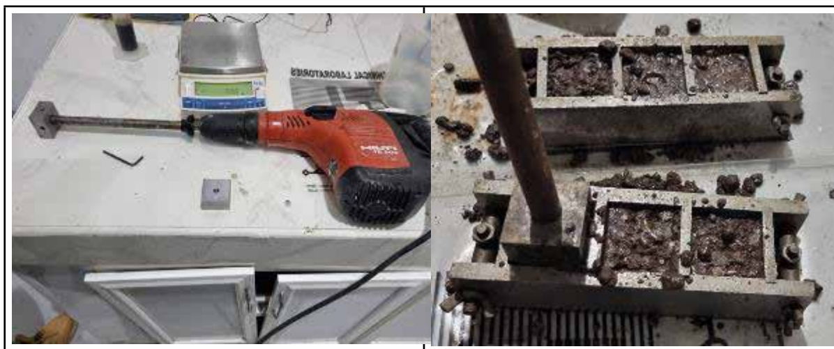
Figure 5-5 Compaction of the concrete cubes using a vibrating hammer
