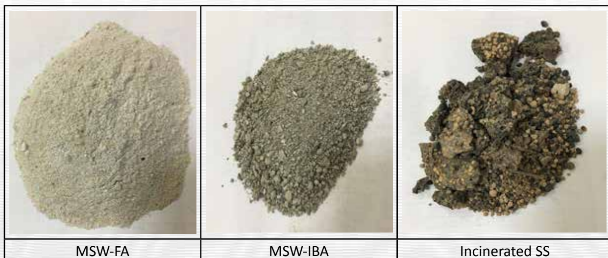
Figure 3-1 Incinerate waste of municipal solid waste fly ash (left) bottom ash (middle) and incinerated sewage sludge (right)
