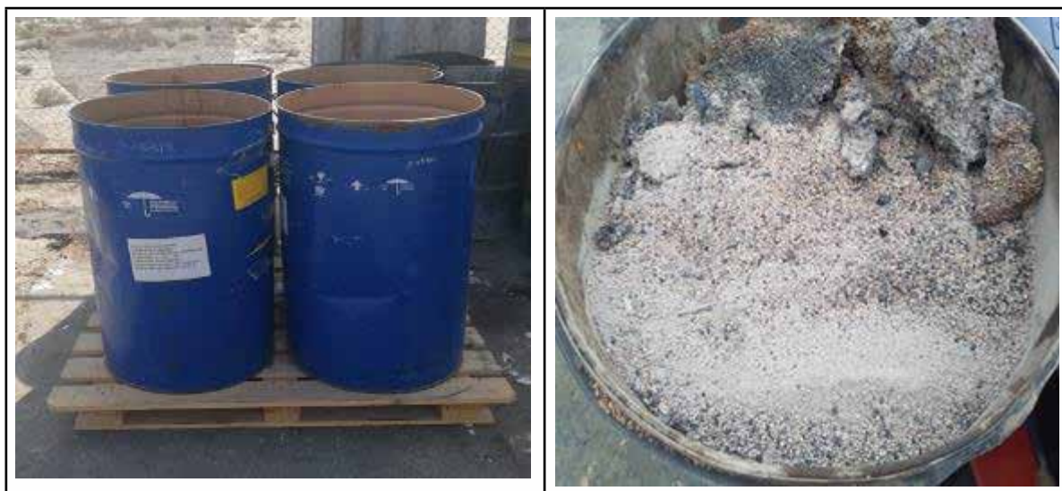
Figure 2-4 SS drums with a top view of the incinerated sludge
