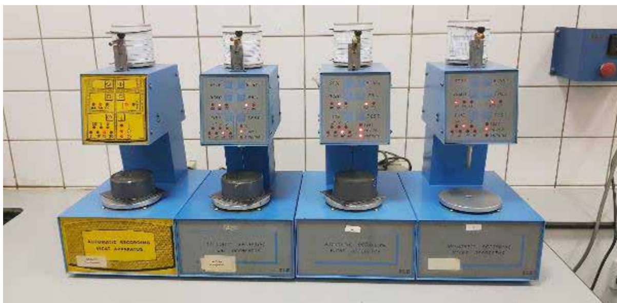
Figure 3-8 Setting time measurements of cement paste (Vicat equipment)
