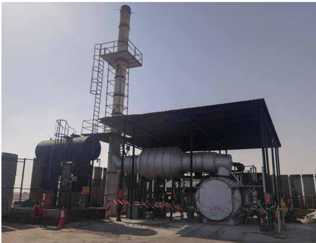
Figure 2-3 Incineration plant used for the sewage sludge
