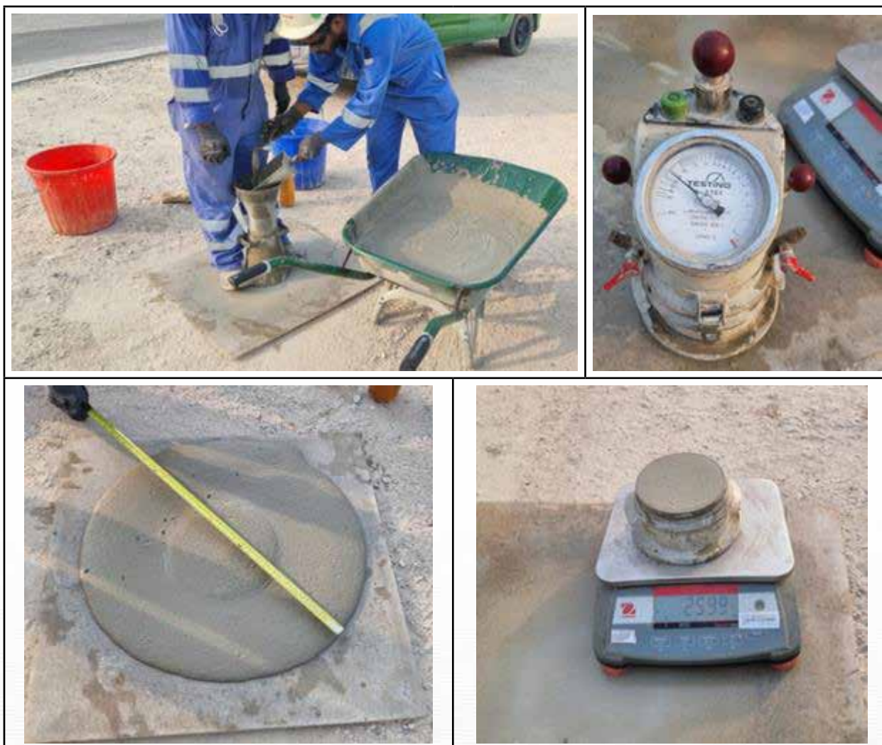
Figure 7-13 Site testing of fresh FC of workability, density, and air content
