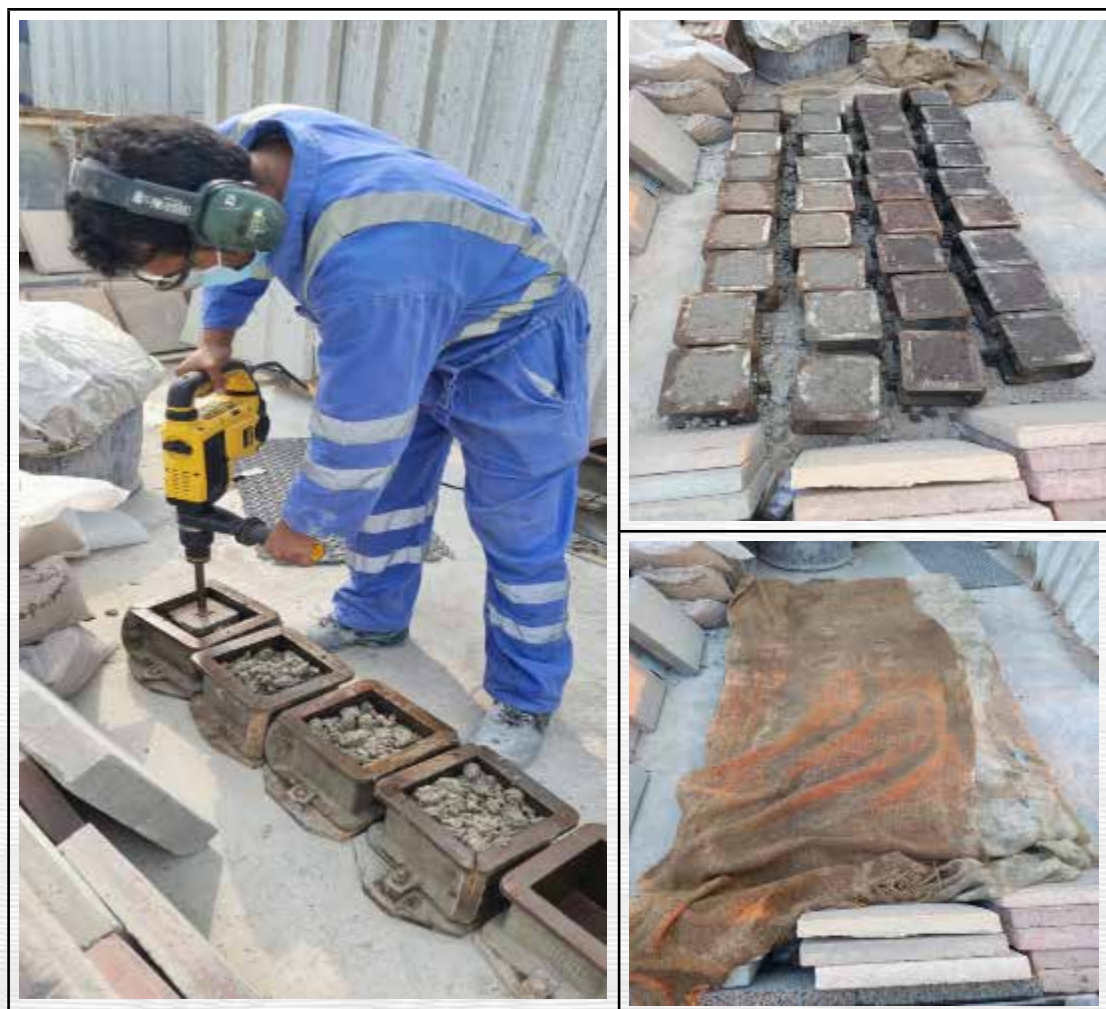
Figure 5-19 Compaction and curing of CBM cubes
