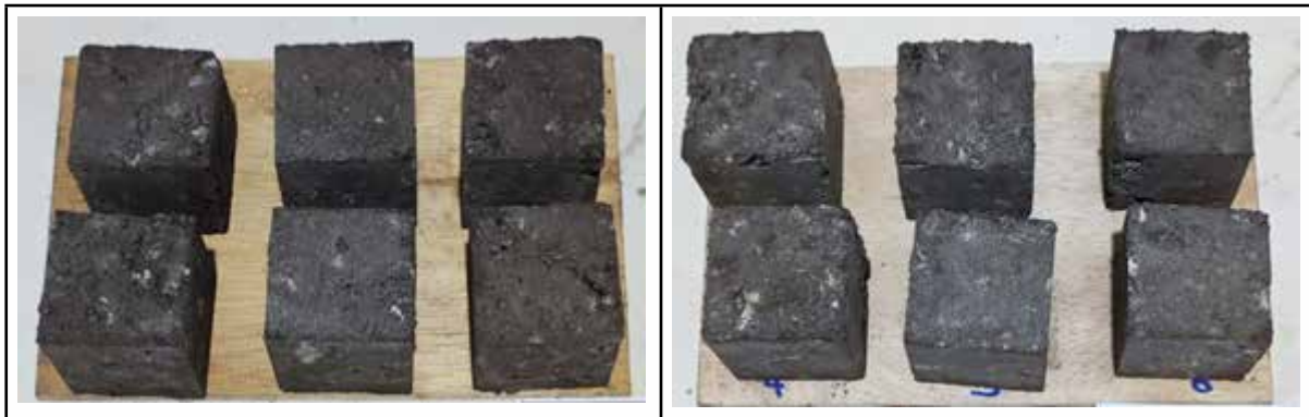
Figure 5-6 Cured cubes after 7 days, SSA-PC (left) and SSA-10CKD (right)
