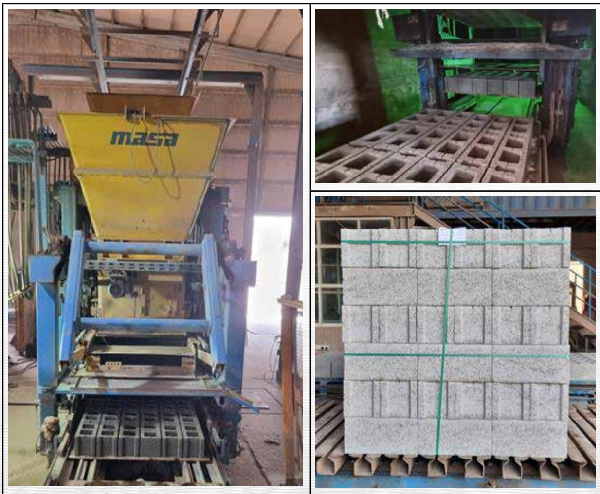
Figure 7-2 Production of concrete blocks, pressure machine (left), curing and final products (right)
