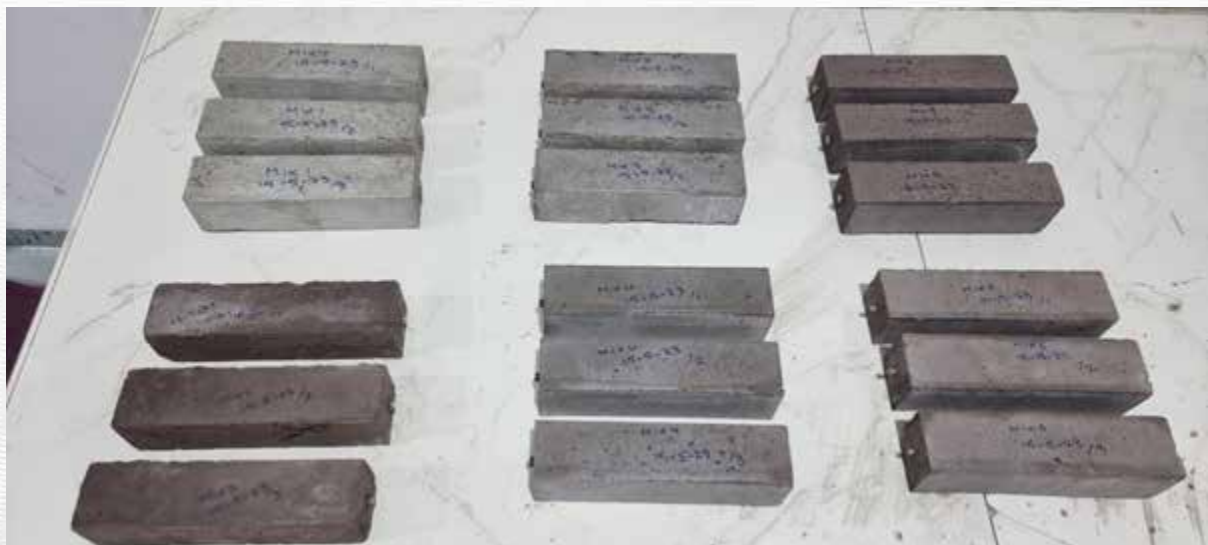
Figure 6-5 Mortar prisms used for the drying shrinkage testing
