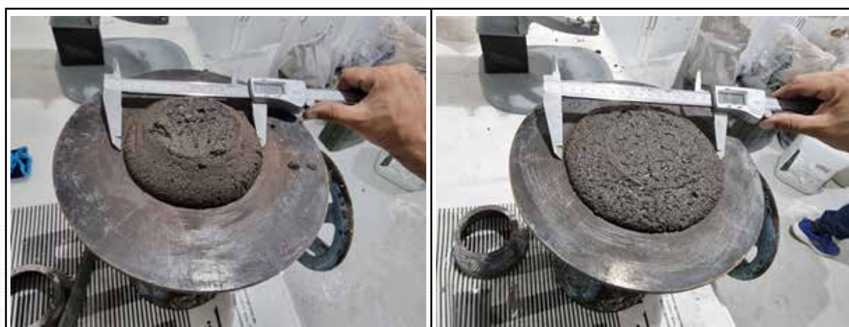
Figure 4-11 Flow table of SSA 8-1.0 (left) and SSA 6-1.0 (right)
