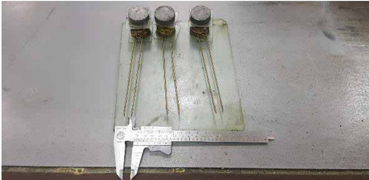
Figure 3-10 Soundness test of cement paste specimens
