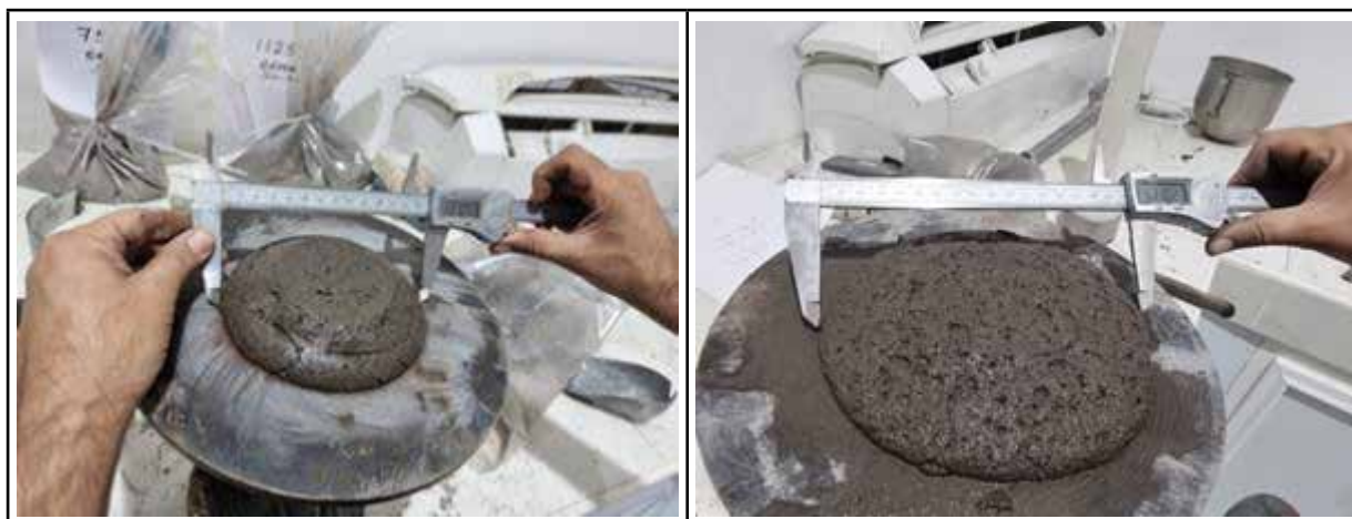
Figure 4-10 Flow table of SSA 8-1.5 (left) and SSA 6-1.5 (right)
