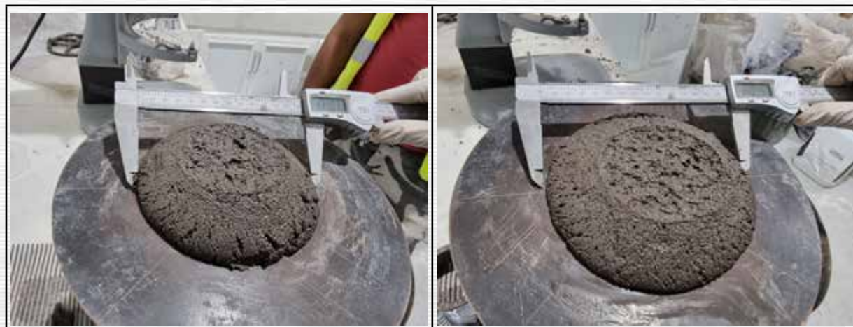
Figure 4-12 Flow table of SSA 8-0.5 (left) and SSA 6-0.5 (right)
