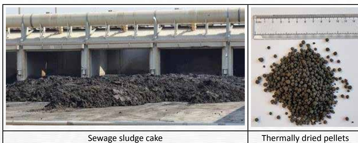
Figure 2-1 Sewage sludge cake (left) and thermally dried sludge pellets (right)
