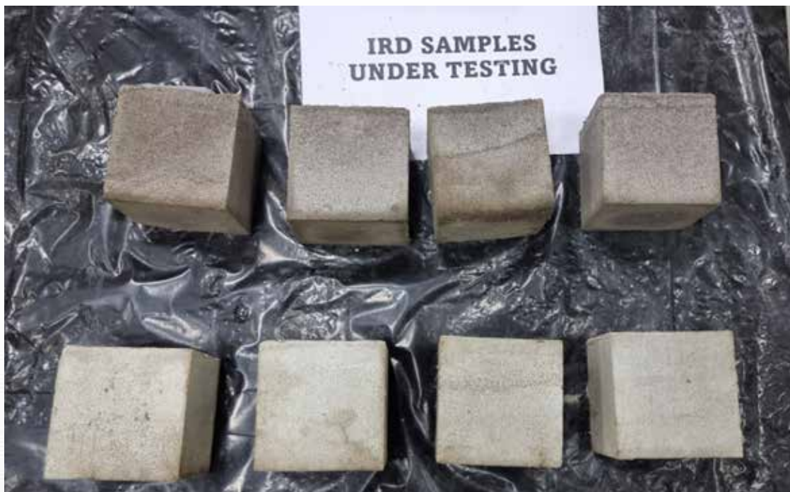
Figure 7-14 Concrete cubes for density and strength measurement
