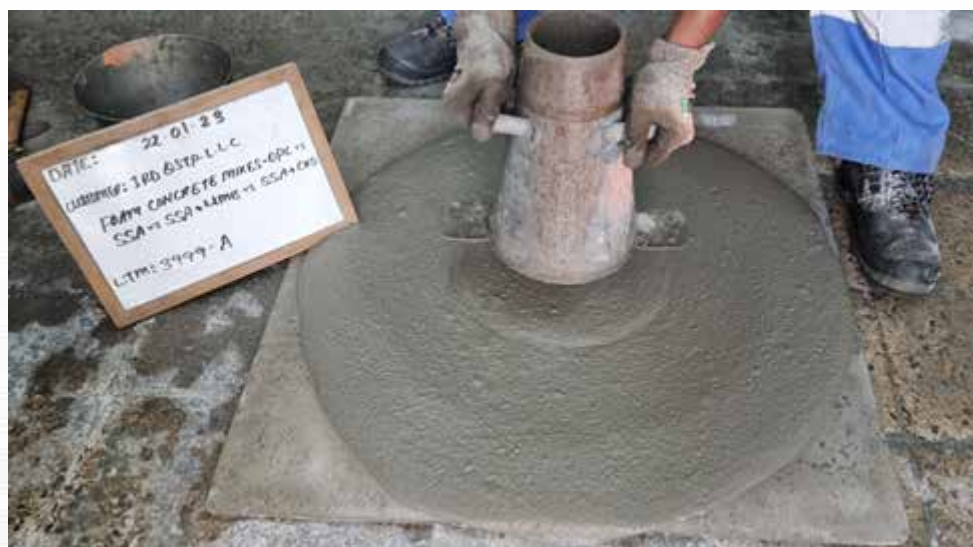
Figure 5-12 Workability of foamed concrete
