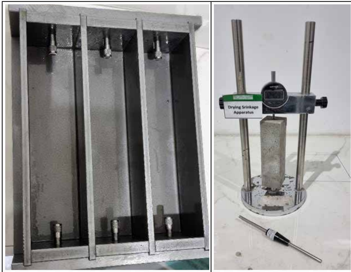
Figure 6-4 Shrinkage moulds and testing apparatus
