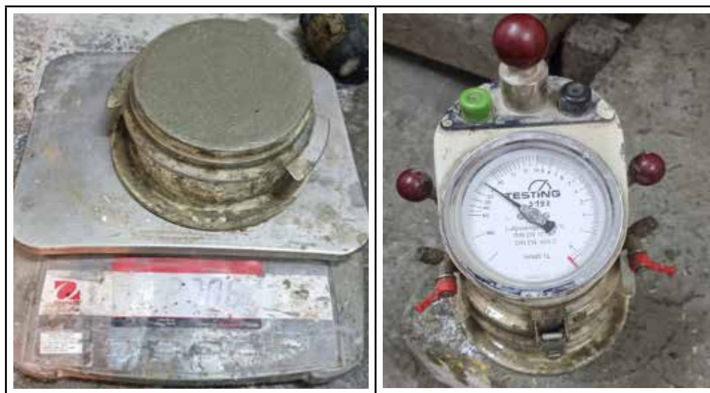
Figure 5-11 Wet density (left) and air content (right) testing
