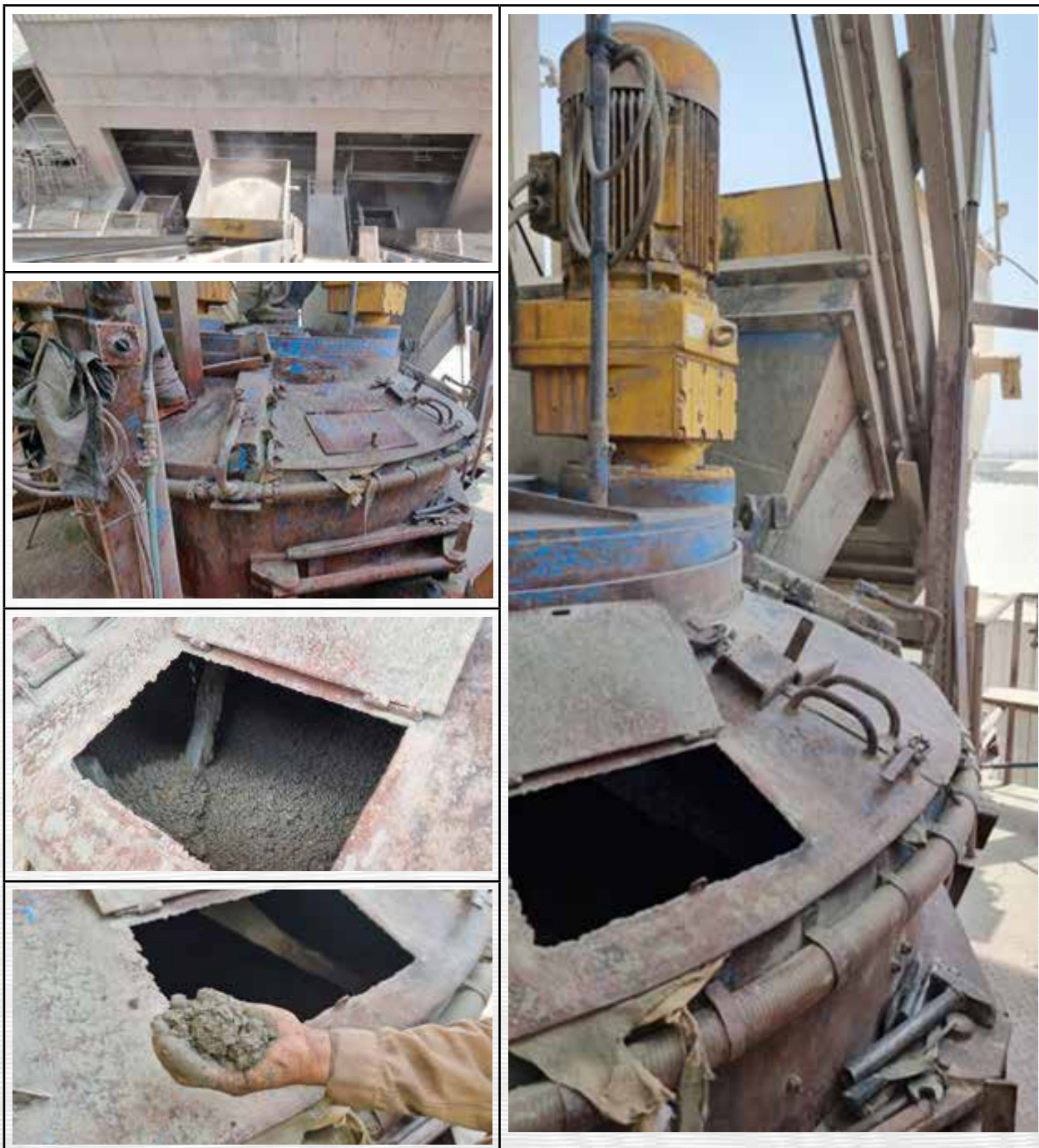
Figure 7-1. Mixing of the concrete block materials
