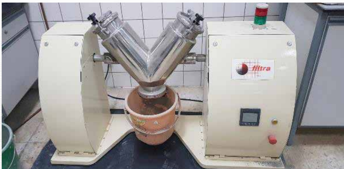
Figure 3-7 A rotating V-shape mixer for homogeneous cement paste specimens
