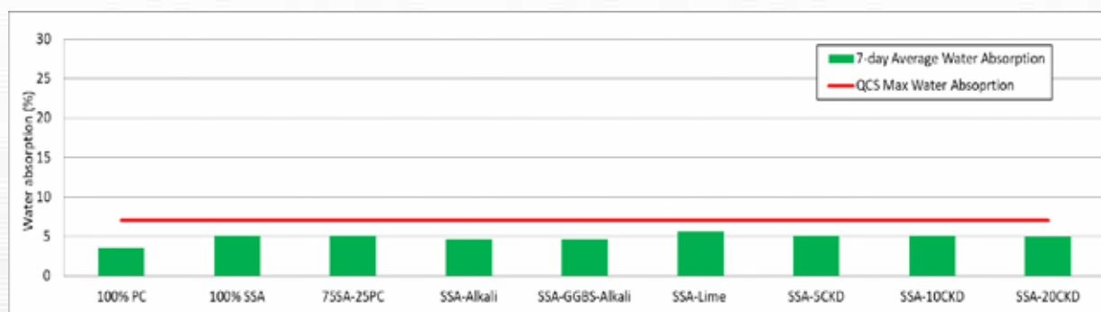
Figure 5-8 Water absorption of the concrete mixtures at 7 days
