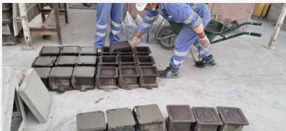
Figure 5-13 Cube preparation for the different FC mixtures
