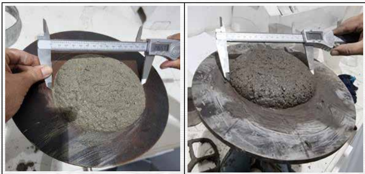
Figure 4-3 Flow table testing of PC (left) and SSA (right)
